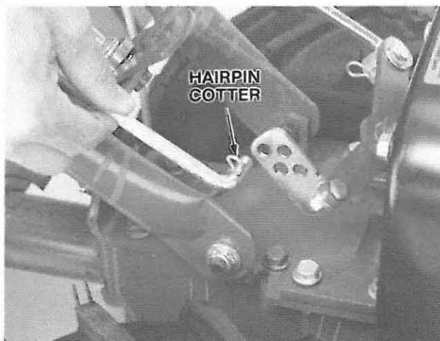
Photo 2-9: Installing the Forward Clutch Rod.
