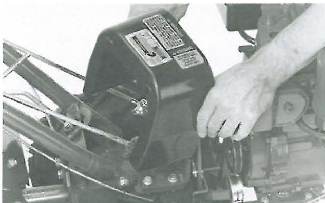
Photo 4-5: Removing Belt Cover.
