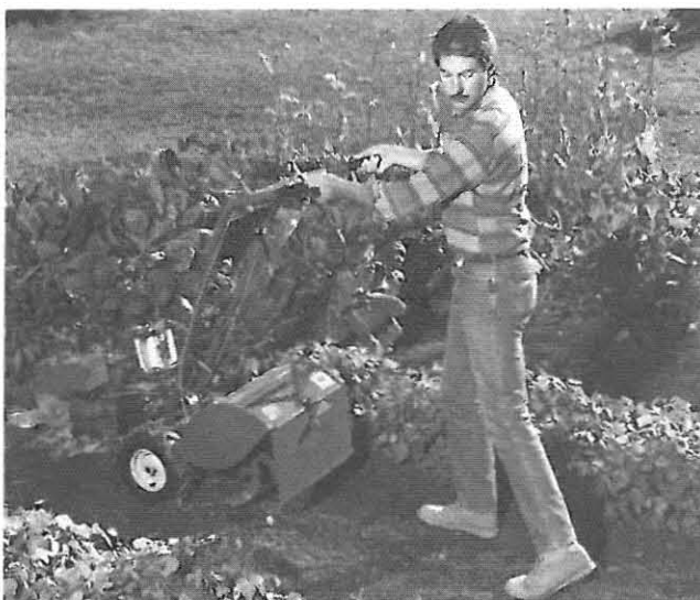
Photo 4-17: To turn around in cramped quarters, move close to obstacle, then put the tiller in Reverse while lifting up on the handlebars (to raise the tines out of the soil) and turning the tiller.
