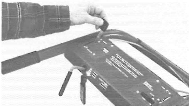
Photo 3-2: The Wheel Gear Lever in "ENGAGE" position. Econo-Horse and Pony Models only.
