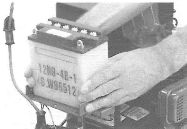
Photo 2-23: Installing the Battery.
