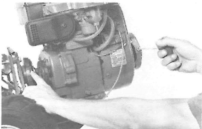
Photo 5-15: Slipping the Forward Drive Belt off the engine-driven pulley.
