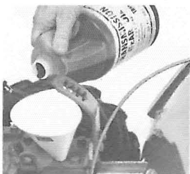
Photo 5-4: Adding gear oil to transmission. Stop when oil exits from check hole at the side.
