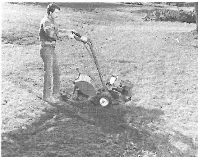
Photo 4-3: Use the wheels as a pivot point to balance the engine and tines. Push the handlebars sideways to move the tiller in the direction of the turn, and continue up the next row. Shown is the Econo-Horse Model tiller.
