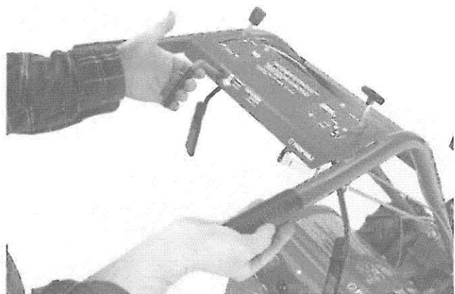
Photo 3-4: The Maneuvering Clutch.
