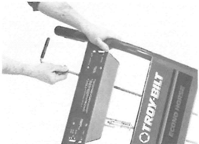
Photo 2-5: Removing the Maneuvering Clutch Lever from the handlebars.
