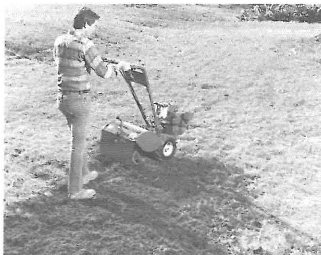
Photo 4-2: When you reach the end of a row, slow the engine down and lift up on the handlebars to raise the tines from the soil. The Econo-Horse Model is shown.
