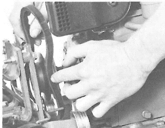
Photo 5-19: Installing the Forward Drive Belt.
