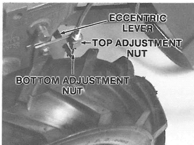
Photo 5-27: Adjusting Wheel Gear Cable. (Econo-Horse and Pony Models only.)
